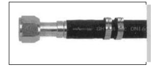
Step 5. Snap the cage into the groove on the nipple. The arms should extend over the hose length. When the cage has been correctly installed in the cage groove, the cage will be able to rotate in the groove. This step MUST be performed to ensure:
